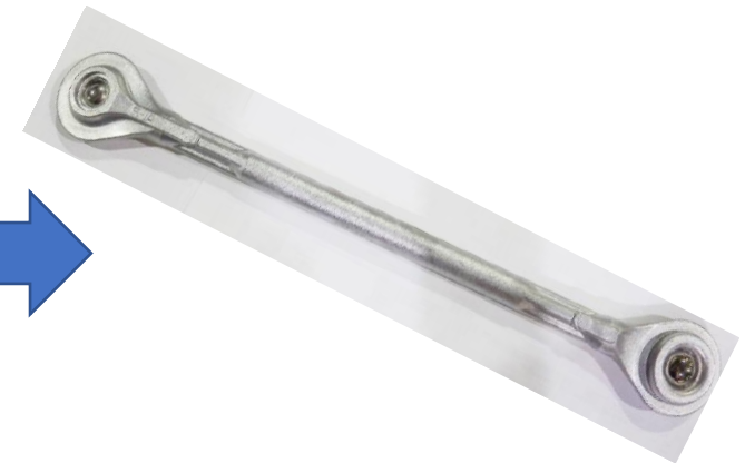
Excess material is cut off and...voila! A completed casting!
